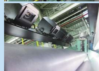
Automated defect detection equipment installed on the 1600-millimeter leveling line as part of our efforts to improve customer satisfaction
