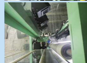
Automated defect detection equipment on the 1250-millimeter leveling line. Defect detection is carried out according to customer requests.
